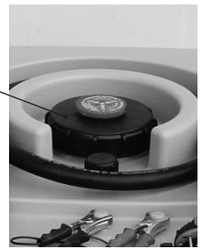
Fig. 5.4.2: Filling opening on 4601 / 6001 tank
